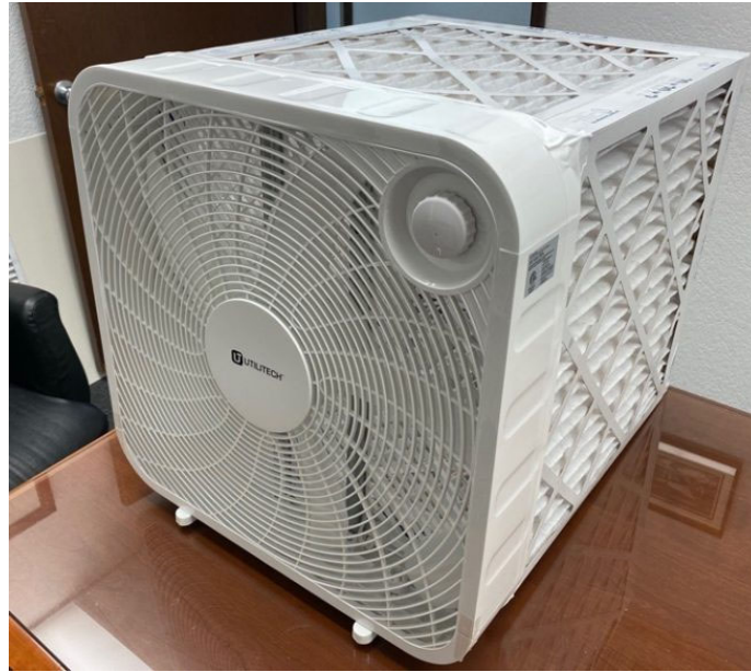
A Corsi box (pictured) is a low-cost, DIY indoor air filtration solution that consists of one box fan plus five filters arranged in a cube.
